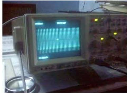
Fig. 6 Measured Result of Fiber Transmit Waveform
