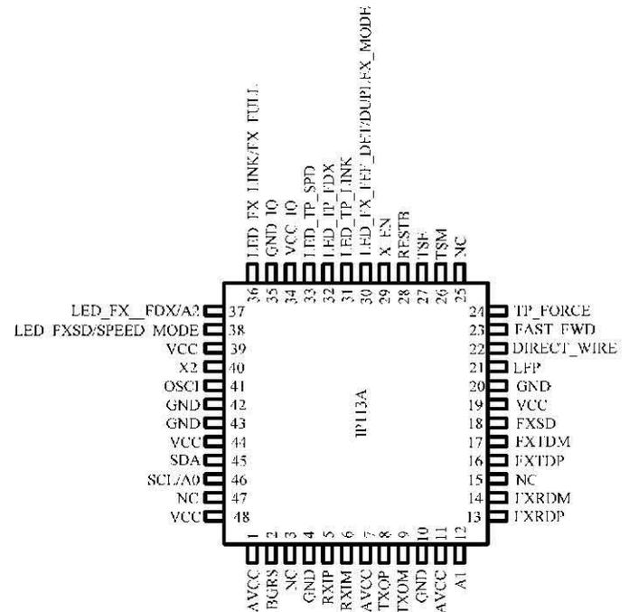
Fig. 2 Pin Diagram of IP113A
