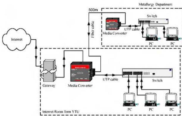
Fig. 3 Proposed System of Media Converter
