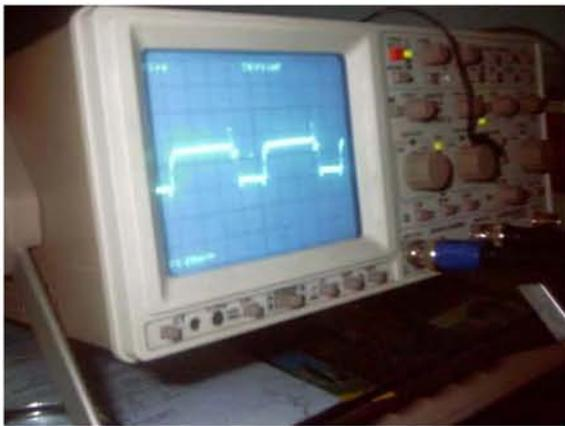
Fig. 4 Measured Result of Twisted Pair Transmit Waveform
